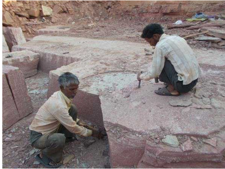
Figure 4: Process of breaking stone through chisel-hammer
